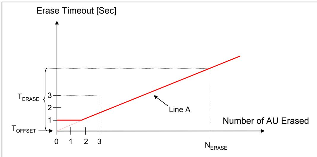
Figure 4-17: Example Erase Characteristics (Case 1  $T_{OFFSET}=0$ )
