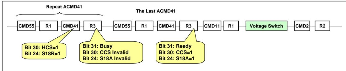
**Figure 4-5 : ACMD41 Timing Followed by Voltage Switch Sequence**
