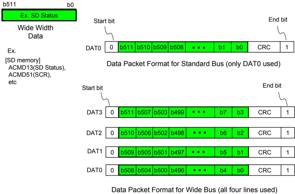
**Figure 3-7: Data Packet Format - Wide Width Data**
