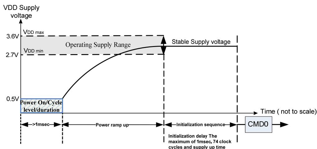
**Figure 6-2 : Change of Figure for Power Up**
