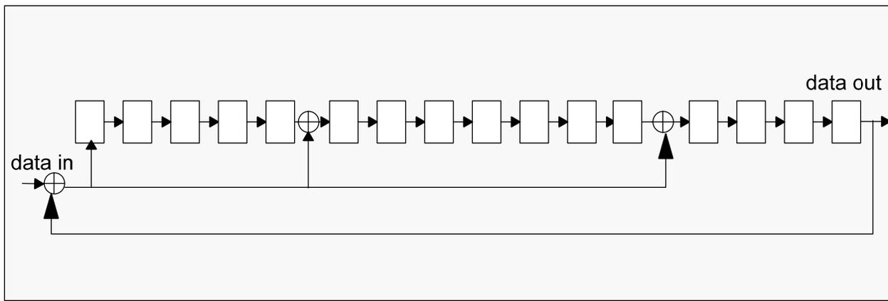
**Figure 4-13: CRC16 Generator/Checker**
