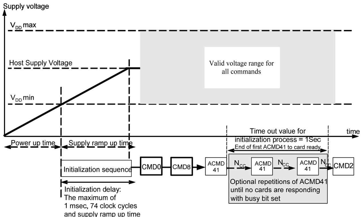
**Figure 6-1: Power-up Diagram**
